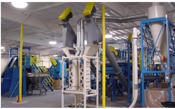
MBA Polymers' pre-processing line.
