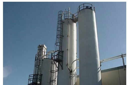
Big silos are needed for storage and blending to ensure consistent products.
