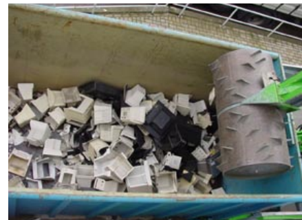
Pre-processing of electronic scrap.
